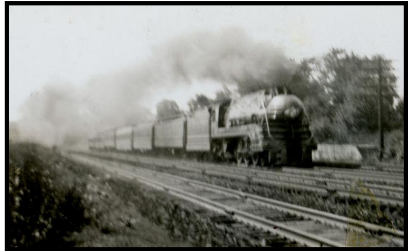
ABOVE: The westbound Asa Packer cruises by the old Hokendauqua station platform on track 1. From left to right, tracks were numbered 3, 4, 1, 2. Tracks 3 and 4 were for freight trains, while 1 and 2 were for passenger trains. This train, Train 25, usually passed through Hokendauqua by 1000.
